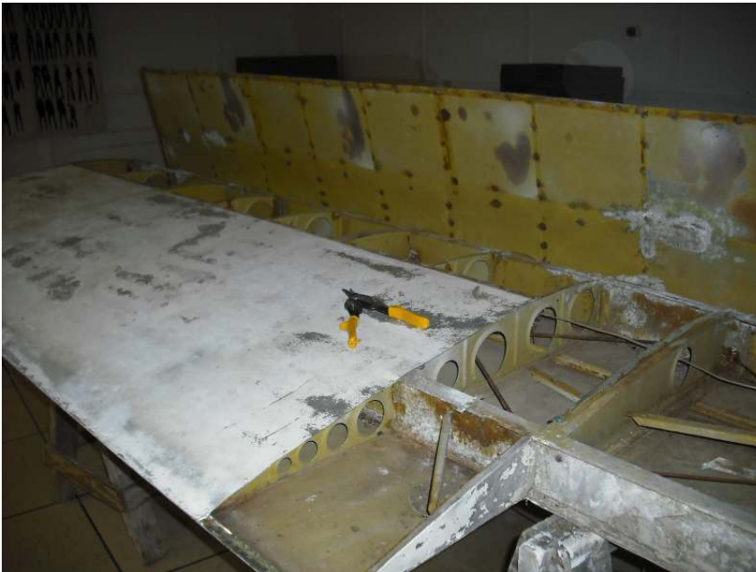
Waiting conduit and then riveting back together
